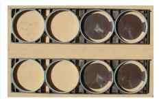
Step 2: Place a ring on each cavity, positioning the ring with the notch side down. If the ring is positioned properly, it will fit down snug and flush without force.
