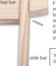
Finally (see pic at left) add 1 more nail on each end of the top board, that will go at an angle through the side board into the top board to provide a little extra sturdiness for when you are pulling frames.
